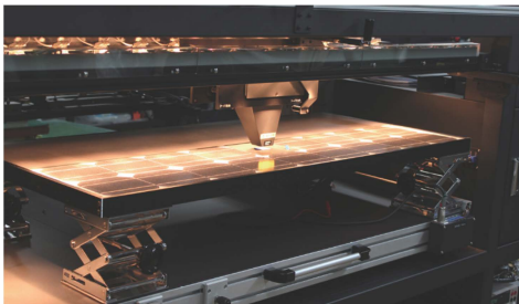
The photo shows the CEP-M1000 perform the spectral response measurement.
