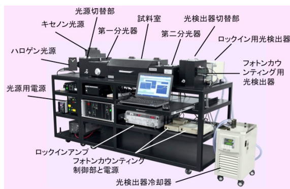
Fig.1 Photograph of developed spectrophotometer
